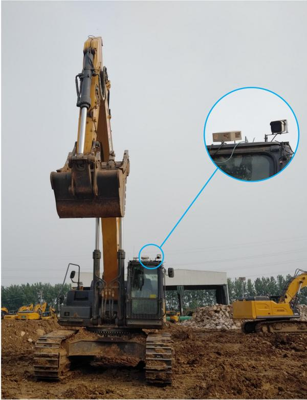
Figure 1. The autonomous walking excavator which is equipped with a cabin-mounted LiDAR(Livox Mid100) and a HIK web camera.
